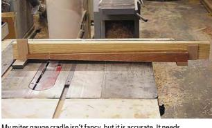
My miter gauge cradle isn't fancy, but it is accurate. It needs to hold the centerline of the leg parallel to the saw table during the cut. Don't worry about how high off the table the cradle holds the leg. Adjusting the blade height will set the cut's depth perfectly.
