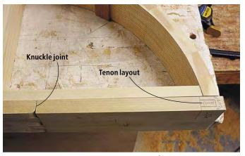
With the length of the two swing legs determined ( $^{1}/_{4}$ " beyond the apron corner) you're ready to lay out the tenon location on the end of each piece. Then cut the tenons and the corresponding mortises in the legs.
