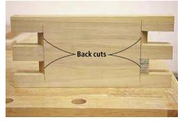
To allow enough room for the swing rails to open, on the back side of the center rail draw a line <sup>3</sup>/<sub>4</sub>" behind the shoulder cut at the saw. With a hand saw cut small cuts to that line while maintaining the front edge shoulder. With the cuts made, chisel away the waste.
