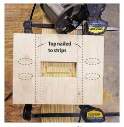
I make my routing template using  $^{1}/_{2}$ " Baltic birch plywood. Rather than cut out and clean up a hole, I make my template from four pieces and hold them together with biscuits. This method leaves an accurate opening that is  $1^{5}/_{8}$ " wide x 4" long.
