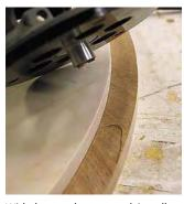
With the template secured, install a <sup>5</sup>/8" straight-cutting bit with a <sup>3</sup>/4"-outside diameter bushing into the router and remove waste material to create the recess for the edge banding.
