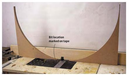
To rout the grooves for the apron stringing, attach the template scraps to a sacrificial fence on your router table. Attach them so that the apron just fits inside the pair. Install a  $^{1}/_{16}$ " straight bit set to an  $^{1}/_{8}$ " height and mark both sides of the bit width on a piece of tape that extends about 5" from the bit. Mark a line that is  $^{3}/_{4}$ " from each end of all the panels of the apron. Set the fence  $^{5}/_{8}$ " from the bit and you're ready to rout.
