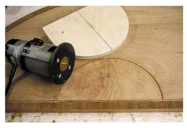
Clamp this template in place, and follow the direction on the inlay kit to cut the area and the matching inlay.
