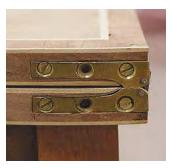
The hinge I used allows the joint to remain loose when moving. This gives the joint space to move without rubbing the two parts of the top together.
