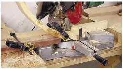
To trim the ends of the apron, patience and accuracy are required. I clamped the apron to my miter saw, carefully checking the squareness of the end mark to the blade before making the cut.
