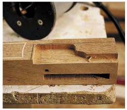
After marking the legs at the meeting point of the apron, remove the legs from the swing rail. Use a router and straight-cutting bit to remove as much of the material as possible. Don't cut past the lines. Finish up any remaining material with a sharp chisel.
