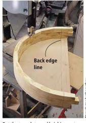
Set the template and bricking onto the guide pin and make a slow, steady cut using a <sup>1</sup>/<sub>2</sub>" skip-tooth blade. The resulting apron thickness is slightly over 1" thick, completing the curved apron.
