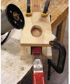
The cradle supports the leg from underneath. The top piece with the oval template is clamped to the box, centering the cut between the top of the leg and the lower edge of the apron as well as the middle of the leg. Note that the orangehandled clamp serves to keep the leg positioned lengthwise in the cradle.
