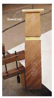
With the oversized veneer panels you should not have trouble placing the veneer panels on the apron. Make sure to roll the panels to smooth any small air bubbles. I use a section of dowel rod for this step.
