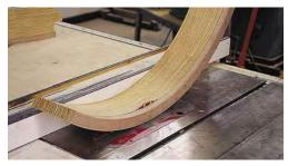
Make your first cut to remove the template piece. Hold the apron as tight as possible against the fence during this step. Then reset the fence to the finished height of the apron, rotate the piece to the opposite edge and make your second cut.
