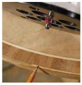
Here I have changed the bearing on a flush-trim bit to allow for a  $^{1}/_{16}$ " cut. You need to run the top and bottom of both the top and the sub-top.
