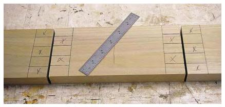
To mark out the knuckle spacing, set one end of a ruler (at zero) on one side of the board and set the 5" mark on the opposite edge of the board. Then transfer each of the inch marks to both ends of the center rail and one end of each swing section.
