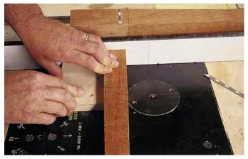
Holding the top of the leg against the fence and the face side toward the table (remember that the face side of the rear or back legs is the side facing outward, opposite of the mortise) make a pass over the bit, cutting the thickness of your inlay.
