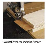
make a first cut on the end of the veneer strip, then slide the veneer out about an 1<sup>1</sup>/<sub>4</sub>" and make a second pass. This creates the first piece of edge band veneer. You will need 22 or more pieces of this curved edge banding.
