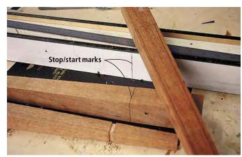
Install a  $^{1}/_{16}$ " bit in the router table and set the fence  $^{1}/_{4}$ " from the bit. Set the bit to cut  $^{1}/_{8}$ " deep. Run the cut on two edges of the face, from the  $^{4}/_{2}$ " line at the top of the leg into the area that was cut for the cuff.
