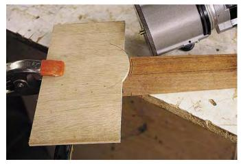
Start the scalloped stringing cut by inserting the bit into one side of the existing cut and move toward the opposite side until it just enters the second side cut. Keep the bushing against the pattern.
