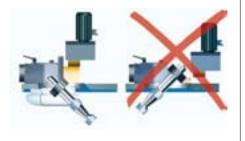
flexibility to the machine's capabilities. Unfortunately, most ordinary machines tilt to the front side, which is a very old design and not considered very safe. There are very few manufacturers whose spindle tilts in the rearward direction, which is the modern and safe operating technique.
